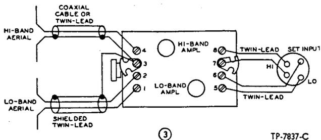
Where only the low band is to be used, make connections as shown in 1, 2, or 3, and remove the high-band amplifier tube.
