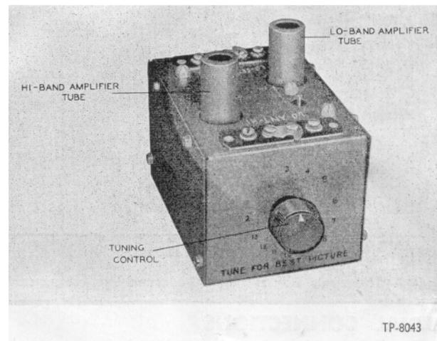
To operate the Booster, set the Booster control to the number of the channel it is desired to receive, and tune in the television station on the receiver in the regular manner. Then carefully readjust the Booster control for the best picture.
