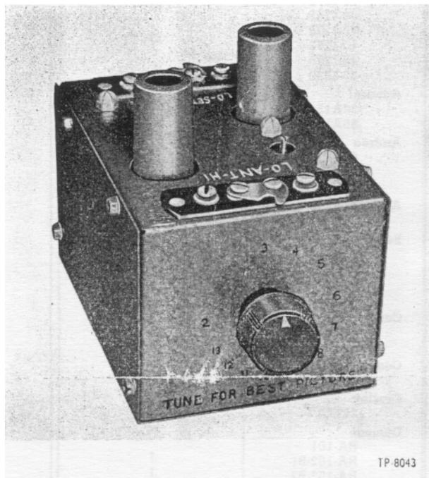
supplied with either of two types of cable, one type (Part No. 41-3914) for receivers using a 6K6, 6V6, or similar octal tube, the other type (Part No. 41-3913) for sets using 7B5, 7C5, or similar Loktal tube. Plug the adapter end of the cable into the socket from which the tube has been removed, then plug the tube into the adapter.
