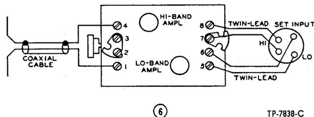
When the Booster is to be used with television receivers having only a single input, the output connections from the Booster to the receiver should be made as shown below.
